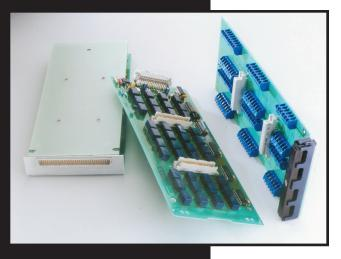
The Model 7011 40-channel multiplexer has four independent banks of 1×10 switching. Each channel is 2-pole. These four banks can be combined for a wide variety of switching configurations—for example, dual 1×20, or 1×10 and 1×30, or one large 1×40. The 7001 mainframe can automatically configure the 7011 to switch 4-pole signals by combining channel pairs. This gives you a dual 1×10 4-pole multiplexer or a single 1×20 4-pole multiplexer.
